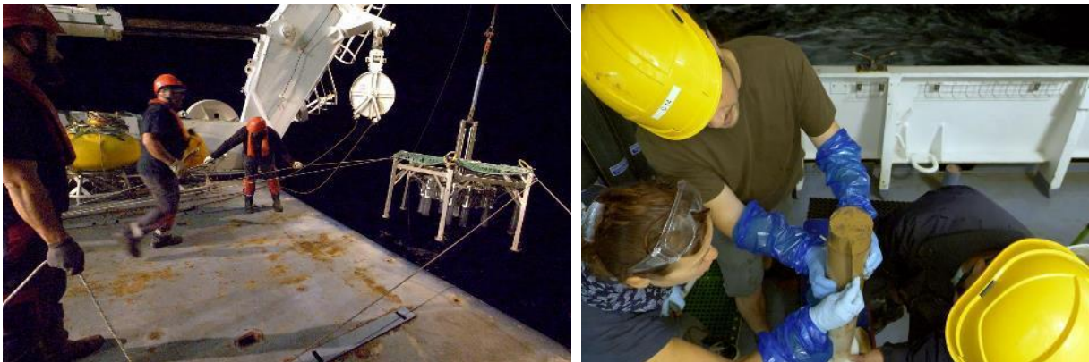
Figure 35. Launching of the Octopus Multicorer at night (left). Slicing a core (right).
