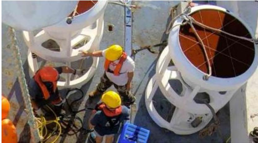
Figure 29. The 2 PPS5 to be deployed at the long station during TONGA. The bottles that collect the material are at the base of the structure.
