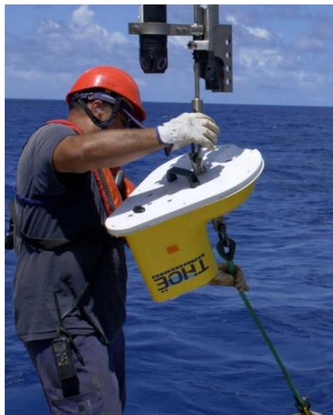
Figure 33. *A THOE instrument installed on the TONGA fixed mooring.*
