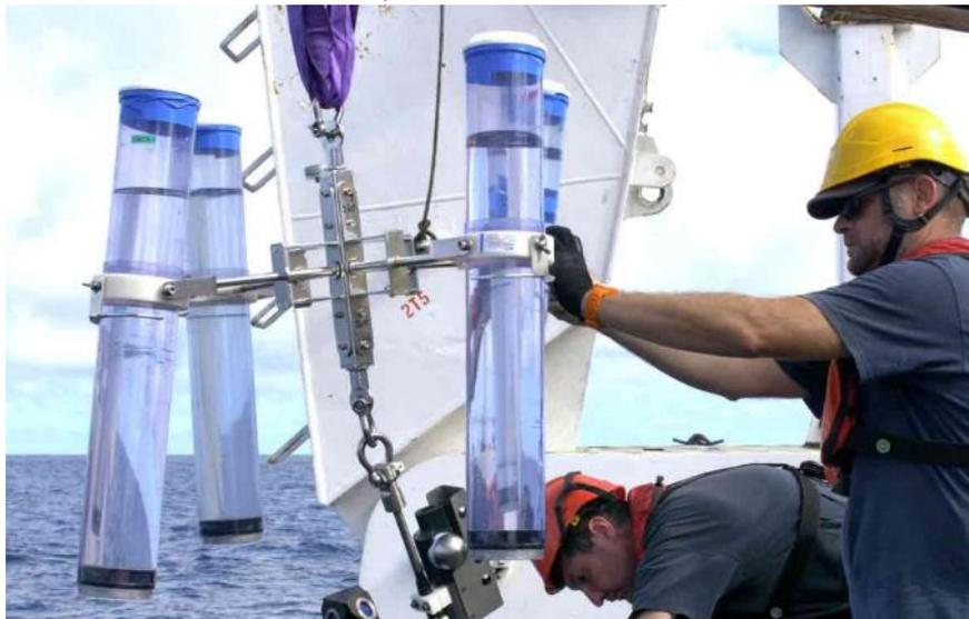
Figure 30. Acrylic traps deployed at long stations 5 and 10 during TONGA
