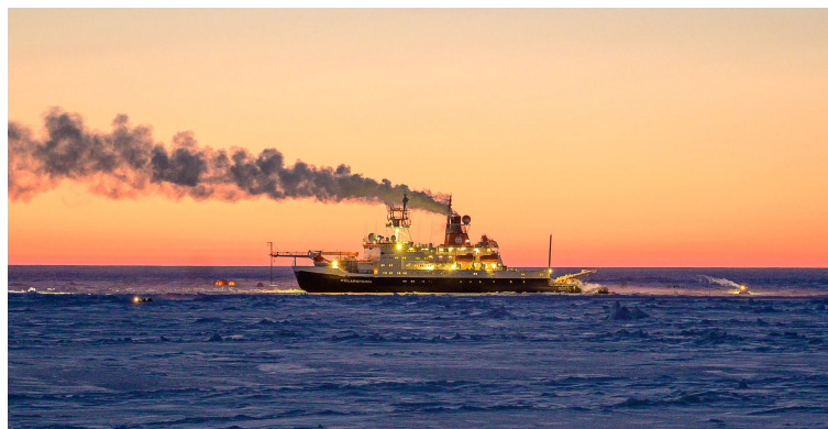
Figure A5. A situation when the wind was coming from the stack's direction and the exhaust plume went directly over the Swiss Container , but due to the surface inversion no pollution spikes were measured in the Swiss Container . The container was located at the bow of the ship, below the crane (left-hand side in this picture). Photo credit: Ivo Beck.
