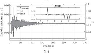
FIG. 12. IR of loudspeaker 6 in the simulated room (a) after 5 s and (b) after 60 s. Gray denotes true IR, and black denotes estimated IR with MISO-AS ( $\kappa=0.1,\,\gamma=0.01$ ). A zoom on the beginning of the IRs is proposed. Errors  $\epsilon$  at the end of simulation are also given at the bottom of the graphs (corresponding scale on the right).
