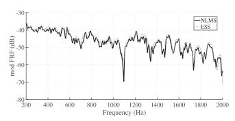
FIG. 16. FRF (magnitude) of loudspeaker 1 in the semi-anechoic chamber. Gray denotes measured with ESS technique, and black denotes estimated with NLMS ( $\tilde{\mu}=0.1$ ) after 60 s.
