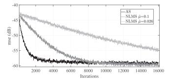
FIG. 6. Learning curves for MISO-NLMS and MISO-AS algorithms. Gray lines: are MISO-NLMS, and black line is MISO-AS. For MISO-NLMS, two different initial values of  $\tilde{\mu}$  are considered. For MISO-AS,  $\kappa=0.1$  and  $\gamma=0.01$ .
