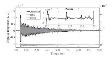
FIG. 19. IR of loudspeaker 8 in the laboratory room. Gray denotes measured with an ESS signal, and black denotes estimated with Autostep after 6 min ( $\kappa=0.01, \gamma=10$ ). A zoom on the beginning of the IRs is proposed. Error  $\epsilon$  is also given at the bottom of the graph (corresponding scale on the right).
