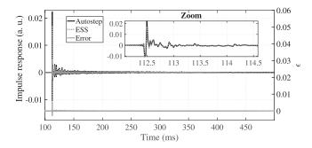
FIG. 18. IR of loudspeaker 1 in the laboratory room. Gray denotes measured with an ESS signal, and black denotes estimated with Autostep after 6 min ( $\kappa = 0.01$ ,  $\gamma = 10$ ). A zoom on the beginning of the IRs is proposed. Error  $\epsilon$  is also given at the bottom of the graph (corresponding scale on the right).
