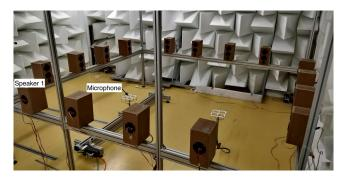
FIG. 13. (Color online) Experimental setup in the semi-anechoic chamber.
