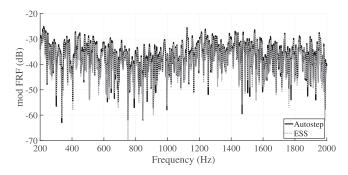
FIG. 21. FRF (magnitude) of loudspeaker 8 in the laboratory room. Gray denotes measured with ESS technique, and black denotes estimated with Autostep after 6 min.
