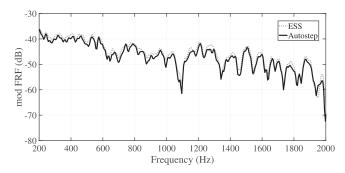
FIG. 15. FRF (magnitude) of loudspeaker 1 in the semi-anechoic chamber. Gray denotes measured with ESS technique, and black denotes estimated with Autostep after 60 s.
