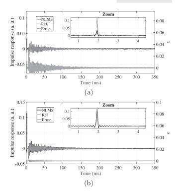
FIG. 9. IR of loudspeaker 1 in the simulated room (a) after 5 s and (b) after 60 s. Gray denotes true IR, and black denotes estimated IR with MISONLMS ( $\tilde{\mu}=0.1$ ). A zoom on the beginning of the IRs is proposed. Errors  $\epsilon$  at the end of simulation are also given at the bottom of the graphs (corresponding scale on the right).
