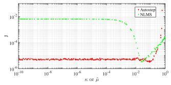
FIG. 5. (Color online) Cost function, J, as a function of  $\kappa$  (for  $\gamma=0.01$ ) or  $\tilde{\mu}$ . Green dots are points where J is calculated for NLMS, and red diamonds are points where J is calculated for Autostep. Minimum values of J are  $3.15\times 10^{-6}$  for  $\tilde{\mu}=2.6\times 10^{-2}$  and  $3.19\times 10^{-6}$  for  $\kappa=9.11\times 10^{-2}$ .
