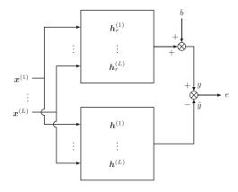
FIG. 1. Block diagram of the adaptive filtering problem, showing (upper block) real (unknown) IRs,  $h_r^{(l)}$  (where r is the subscript for real) and (lower block) recursively estimated IRs,  $h^{(l)}$ . Outputs are such that y is the measured output signal corrupted by additive noise b, and  $\tilde{y}$  is the output sequence of the adaptive filter.
