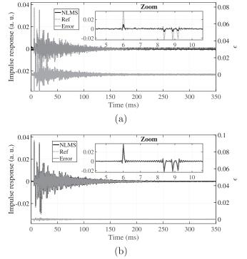
FIG. 10. IR of loudspeaker 6 in the simulated room (a) after 5 s and (b) after 60 s. Gray denotes true IR, and black denotes estimated IR with MISONLMS ( $\tilde{\mu}=0.1$ ). A zoom on the beginning of the IRs is proposed. Errors  $\epsilon$  at the end of simulation are also given at the bottom of the graphs (corresponding scale on the right).
