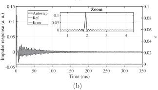
FIG. 11. IR of loudspeaker 1 in the simulated room (a) after 5 s and (b) after 60 s. True IR are in gray, whereas estimated IR with MISO-AS are in black ( $\kappa = 0.1$ ,  $\gamma = 0.01$ ). A zoom on the beginning of the IRs is proposed. Errors  $\epsilon$  at the end of simulation are also given at the bottom of the graphs (corresponding scale on the right).
