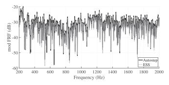
FIG. 20. FRF (magnitude) of loudspeaker 1 in the laboratory room. Gray denotes measured with ESS technique, and black denotes estimated with Autostep after 6 min.
