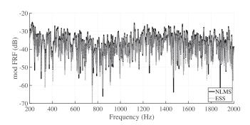
FIG. 23. FRF (magnitude) of loudspeaker 8 in the laboratory room. Gray denotes measured with ESS technique, and black denotes estimated with NLMS after  $6\,\mathrm{min}$ .
