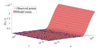
FIG. 2. (Color online) Cost function,  $J(\kappa, \gamma)$ , as a function of  $(\kappa, \gamma)$ . Blue dots are points where J is calculated. Orange surface is Gaussian process regression model. Minimum value of J for  $(\kappa, \gamma) = (0.22, 4.7 \times 10^{-10})$ .
