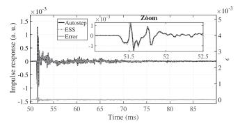
FIG. 14. IR of loudspeaker 1 in the semi-anechoic chamber. Gray denotes measured with an ESS signal, and black denotes estimated with Autostep after 60 s ( $\kappa = 0.01$ ,  $\gamma = 10$ ). A zoom on the beginning of the IRs is proposed. Error  $\epsilon$  is also given at the bottom of the graph (corresponding scale on the right).
