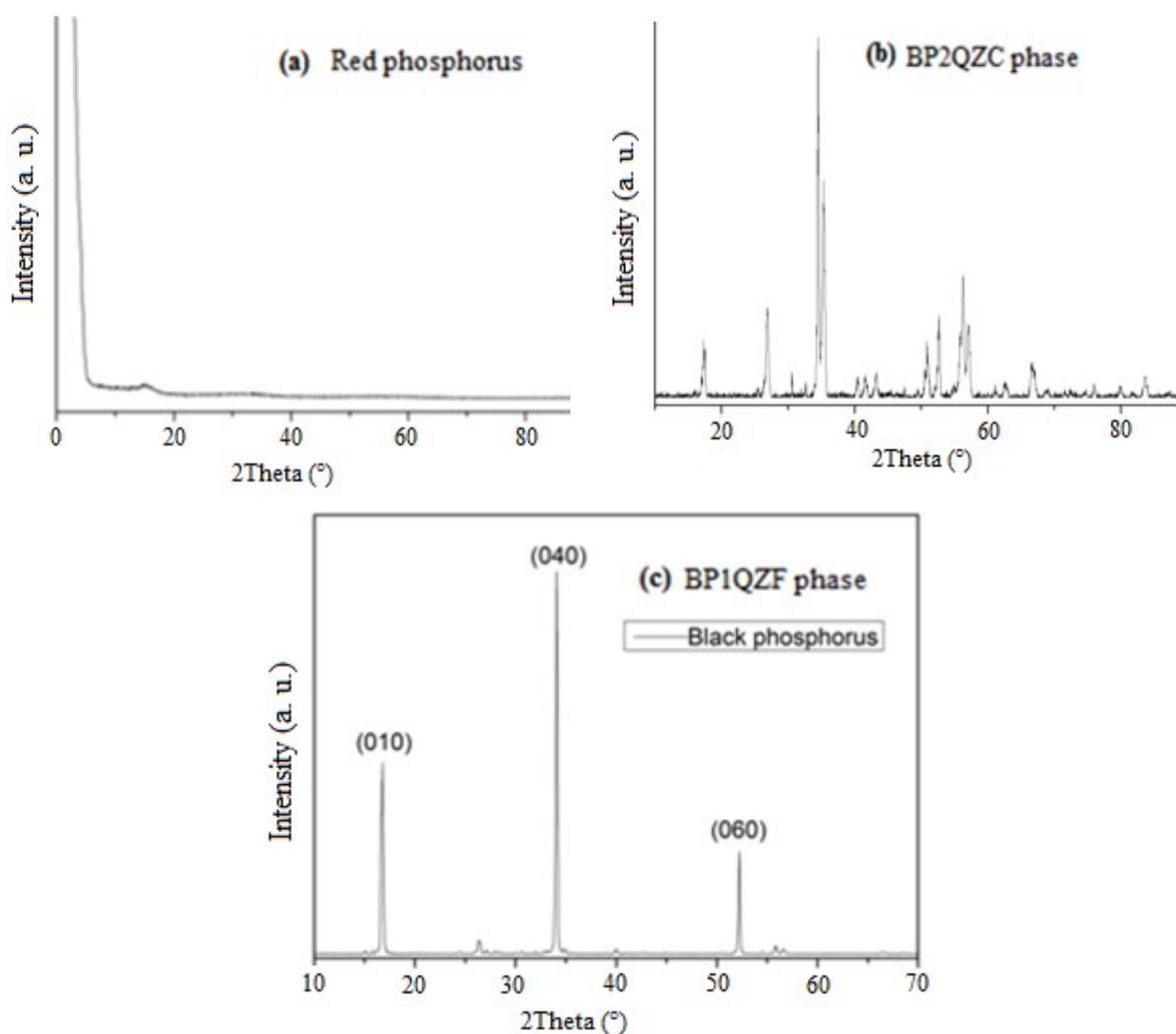
FIG. 1. X-ray powder diffraction: a) red phosphorus, b) BP2QZC phase and c) BP1QZF phase.
