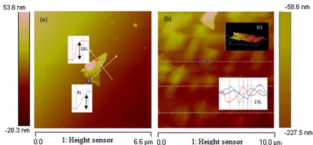
FIG. 6. AFM image of exfoliated BP layers deposited on  $\text{SiO}_2/\text{Si}$  a) lower concentration of BP in NMP (1mg/ml), b) higher concentration (5mg/ml) and c) three-dimensional representation of the surface in (c).
