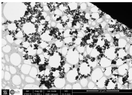
FIG. 5. STEM analysis of exfoliated black phosphorus (13000 rpm).
