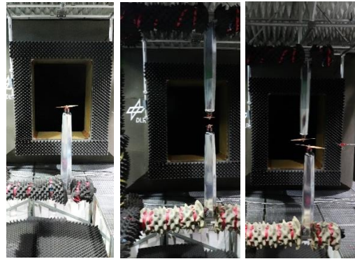
Figure 1 Experimental setup: single rotor (left), coaxial rotors (middle) and tandem rotors (right)
