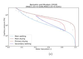
**Figure 9**: Fitted main wetting and main drying curves to the Cement Paste CEM I (material  $N^{\circ}$  2) data from Baroghel-Bouny (2007), and predicted first wetting scanning curve and second drying curve according to the five hysteresis models (one model per subfigure, (a) to (e)).
