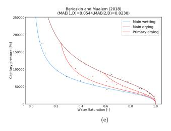
**Figure 11**: Fitted main wetting and main drying curves to the Bentonite MX80 (material  $N^{\circ}$  4) data from Qiao et al. (2021), and predicted first wetting scanning curves according to the five hysteresis models (one model per subfigure, from (a) to (e)).
