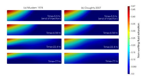
Figure 18: Simulated 2D distribution of the non-wetting fluid (Soltrol-220) saturation at different times (t = 5.5, 6.94, 22.4, 77 hours). (a) Results with the hysteretic model of Mualem (1974). (b) Results with the hysteretic model of Doughty (2007).
