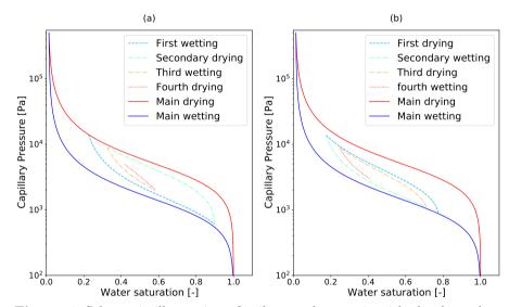
Figure 4: Schematic illustration of soil water hysteresis with the dependent domain theory of Mualem (1984): (a) continuous sequence of scanning curves departing from the main drying curve; (b) continuous sequence of scanning curves departing from the main wetting curve. Idem Van Genuchten parameters of main curves in figure (3).
