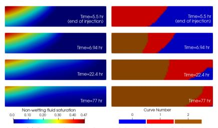
Figure 16: (a) Simulated 2D distribution of the non-wetting fluid saturation at different times by Beriozkin, Mualem (2018) hysteresis model. (b) Flow reversal index numbers where icurve = 0 designates fully saturation state  $(S_l = 1)$ , icurve = 1 designates main drying curve, and icurve = 2 designates the first wetting curve.
