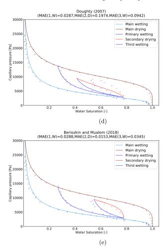
**Figure 10**: Fitted main wetting and main drying curves to the Compacted Sand (material  $N^{\circ}$  3) data from Huang et al. (2005), and predicted scanning curves according to the five hysteresis models (one model per subfigure, from (a) to (e)).
