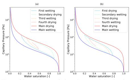
Figure 3: Schematic illustration of soil water hysteresis with the independent domain theory of Mualem (1974): (a) continuous sequence of scanning curves departing from the main drying curve; (b) continuous sequence of scanning curves departing from the main wetting curve.
