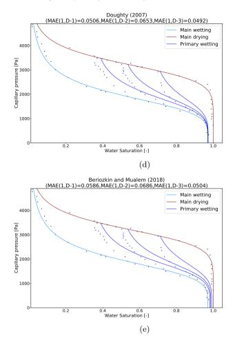
Figure 8: Fitted main wetting and main drying curves to the Dune Sand (material  $N^{\circ}$  1) data from Terleev et al. (2018), and three predicted primary wetting scanning curves departing from the main drying branch, according to the five hysteresis models (one model per subfigure, respectively, from (a) to (e)).
