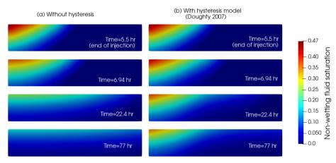
Figure 17: Simulated 2D distribution of the non-wetting fluid (Soltrol-220) saturation at different times ( $t = 5.5, 6.94, 22.4, 77 \ hours$ ). (a) Results from the model without hysteresis. (b) Results with the hysteretic model of Doughty (2007).
