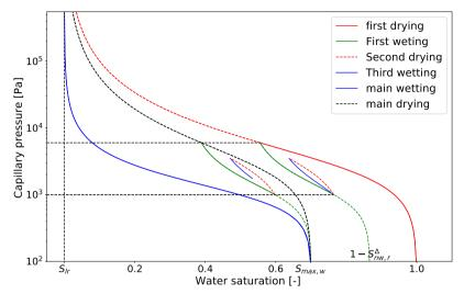
Figure 7: Schematic representation of the hysteresis model of Beriozkin, Mualem (2018), with two parallel sequences of scans departing from the main wetting curve (MWC) and from the first drying curve (FDC).
