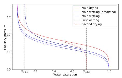
Figure 5: Schematic illustration of soil water hysteresis with the geometrical scaling model of Haverkamp et al. (2002): continuous sequence of scanning curves departing from the main drying curve. Idem VG-parameters in figures (3) and (4).
