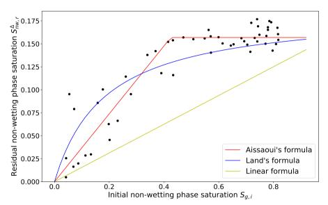
Figure 15: Comparison of non-wetting phase entrapment representations according to the Aissaoui, the linear, and the Land formulae. The points (black dots) represent experimental entrapment data for the Sand 40/50 from Trevisan et al. (2014).
