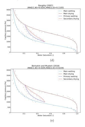
Figure 12: Fitted main wetting and main drying curves to the Hostun Sand (material  $N^{\circ}$  5) data from Lins et al. (2007), and predicted first wetting curve and second drying scanning curve according to the five hysteresis models (one model per subfigure, from (a) to (e)).
