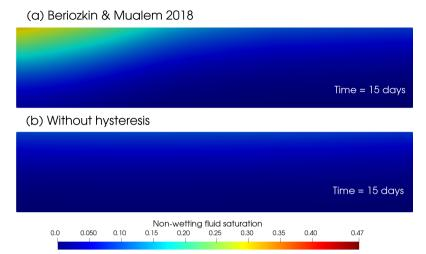
Figure 20: Simulated 2D distribution of non-wetting fluid saturation at the end of the post-injection period  $t = 15 \ days$ . (a) Result with the hysteretic model of Beriozkin, Mualem (2018). (b) Result with the non-hysteretic model.
