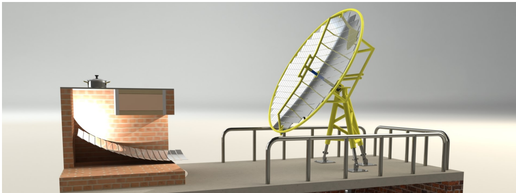
Figure 1: Representation of a solar cooker using a Scheffler reflector and a curved secondary reflector. The Scheffler reflector concentrates the sunlight, while the secondary reflector redirects the concentrated heat flux under the cooking plate.
