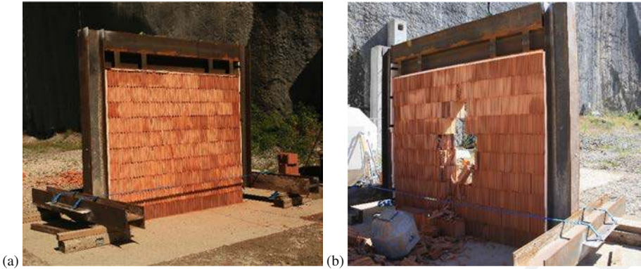
Fig. 2. Full-scale experimental wall #2 prior (a) and after (b) impact.
