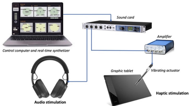
Fig. 2. Set up of the synthesizer device
