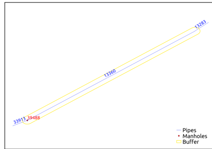
Fig. 6: Example of a pipe with only one node intersecting the buffer area in manholes database, thus one missing extremity.
