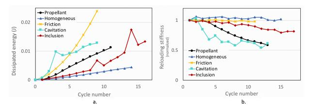
Figure 8: Comparison of the dissipated energy (a) and reloading stiffness (b) evolutions in propellant and HTPB samples, during loading-unloading<sub>1</sub> tests.
