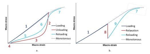
Figure 12: Nonlinear responses of highly filled elastomers under unloading (a) and relaxation (b) cyclic loads.
