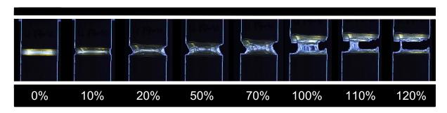
Figure 5: Sequence registered during a monotonous tensile test on a cavitation sample at different strain levels.
