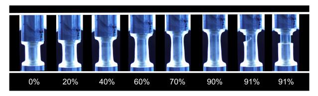
Figure 4: Sequence registered during a monotonous tensile test on a friction sample at different strain levels.
