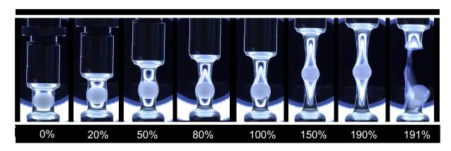
Figure 6: Sequence registered during a monotonous tensile test on an inclusion sample at different strain levels.
