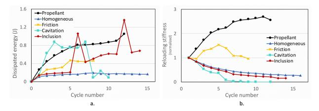
Figure 10: Comparison of the dissipated energy (a) and reloading stiffness (b) evolutions in propellant and HTPB samples, during loading-relaxation tests.
