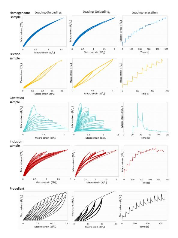
Figure 7: Responses of all HTPB samples to loading-unloading<sub>1</sub>, loading-unloading<sub>5</sub> and loading-relaxation tests. Propellant responses are added for comparison.
