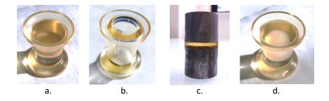
Figure 3: Photographies of the reference (a), friction (b), cavitation (cast between two endplates) (c), and inclusion (d) samples after unmolding.
