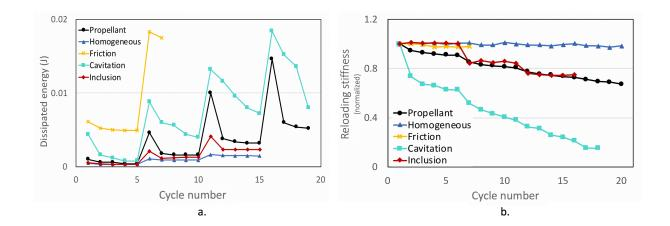
Figure 9: Comparison of the dissipated energy (a) and reloading stiffness (b) evolutions in propellant and HTPB samples, during loading-unloading<sub>5</sub> tests.
