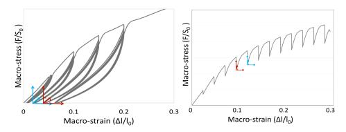
Figure 14: Coordinate systems used to calculate the reloading stiffness after each unloading (a) and relaxation (b) cycle.
