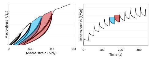
Figure 13: Area calculated to determine the energy dissipated during unloading (a), and relaxation (b) cycles.
