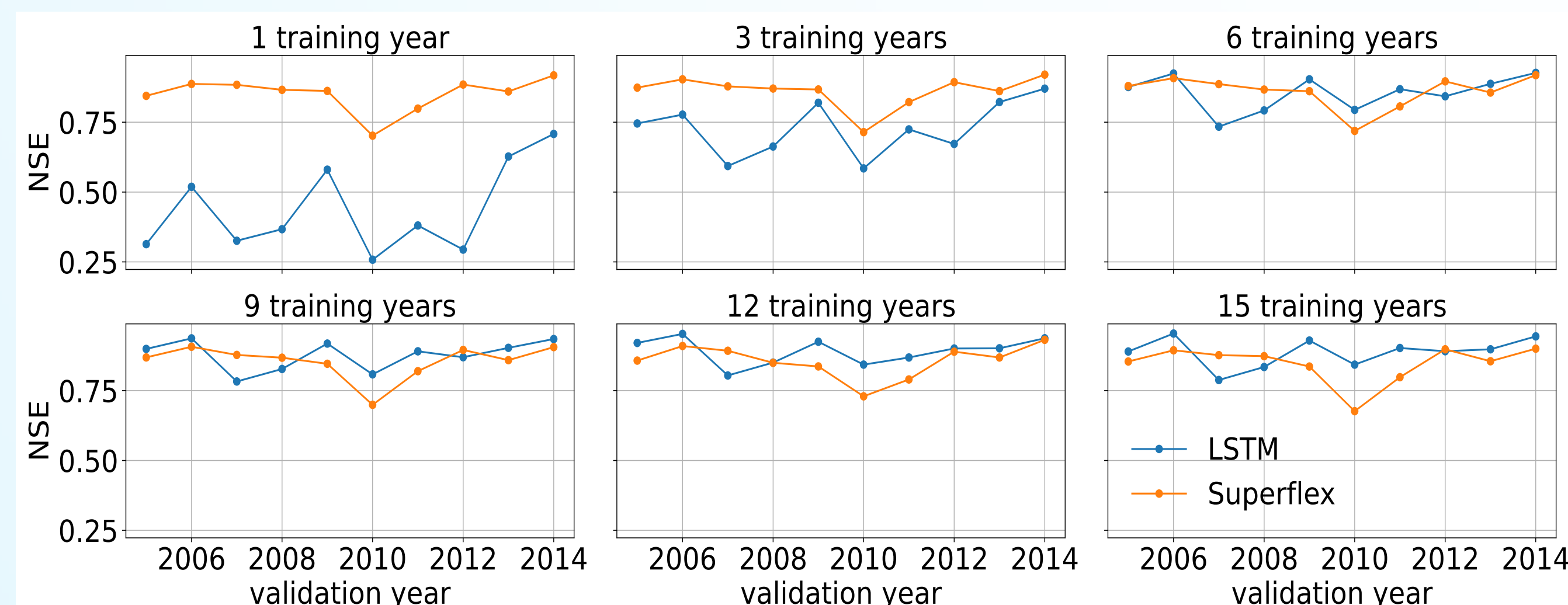
Figure 4 : Average NSE according to validation year obtained by Superflex (orange) and LSTM (blue) models. Each graph represents a fixed number of training years from 1 to 15
