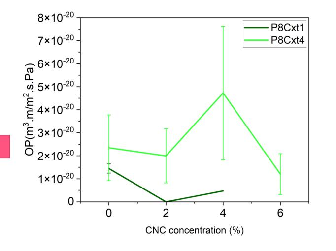
The dry-humid measurements confirm the water vapor sorption results. The addition of CNC in PVA reduce PVA moisture sensitivity. Increasing the CNC concentration reduces the difference between OP in dry and dry-humid. In high relative humidity (80% RH), the water molecules hardly affect the oxygen barrier properties of PVA/CNC coated samples.
