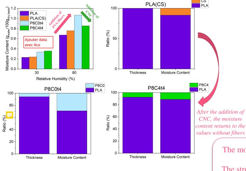
Chitosan (CS), PVA and CNC are hydrophilic polymers. Comparison between PLA and coating ratios shows the high water vapor sensitivity of coating, even with nanometric thicknesses.
