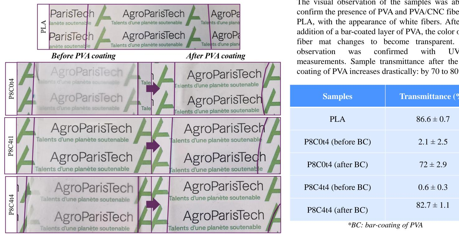
The visual observation of the samples was able to confirm the presence of PVA and PVA/CNC fibers on PLA, with the appearance of white fibers. After the addition of a bar-coated layer of PVA, the color of the fiber mat changes to become transparent. This observation was confirmed with UV-VIS measurements. Sample transmittance after the barcoating of PVA increases drastically: by 70 to 80%.
