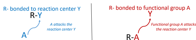
Fig. 1 Reactivity when -R is attached to reaction center Y and when -R is attached to the functional group A.
