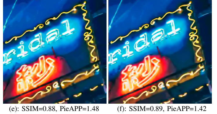
Fig. 11. (a) Original test image (image 3 of the CLIC dataset). The reconstructed ones at 0.2 bpp using: (b) JPEG2000, (c) CNN-LS [23], (d) FCNN-LS-JL-SL [25], (e) FCNN-LS-JL-ML1, (f) FCNN-LS-JL-ML2.
