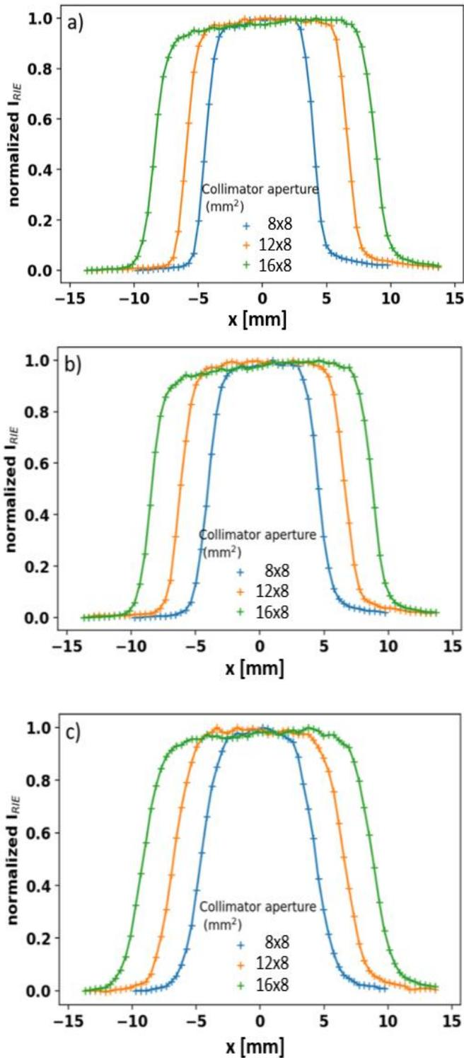
Figure 5: Beam profiles as measured with the Ce-doped rod for all three collimator sizes (blue line: 8×8 mm<sup>2</sup>, orange line: 12×8 mm<sup>2</sup>, green line: 16×8 mm<sup>2</sup>) at a distance of 10 cm (a), 14 cm (b), and 22 cm (c) from the collimator.
