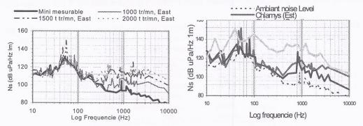
Figure 2: Noise in dB uPa/Hz 1meters from 10 Hz to 10 kHz (logarithmic scale), generated by the Chlamys according to the bearing relatively to the wind direction (East blow). And the second spectral analysis compares the noise of the two boats at 8 knots and the ambient noise of the experiment area.
