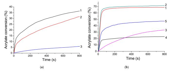
**Figure 7.** Kinetic profiles of the FRP of (a) MAPTMS and (b) MAPTMS 25 wt%/SOA 75 wt% blend mixtures using TXS/Iod  $(0.5\%/2\% \ w/w)$  as the photo-initiating system in laminate and under LED@385 nm (1), LED@405 nm (2), and LED@455 nm (3) after 800 s of irradiation. Photopolymerization under air: curve 4 = irradiation under LED@385 nm and curve 5 = irradiation under LED@405 nm.
