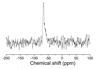
**Figure 6.** Solid <sup>29</sup>Si NMR of the TXS/Iod/DPDO material after 15 min of LED@405 nm irradiation (100 mW/cm<sup>2</sup>).
