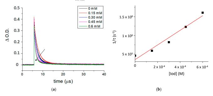
**Figure 4.** (a) Quenching of the transient absorption triplet state of TXS by an increasing concentration of Iod at 640 nm, and (b) the Stern–Volmer plot of  ${}^{3}$ TXS quenching by Iod. Laser excitation at  $\lambda_{355 \text{ nm}}$ .
