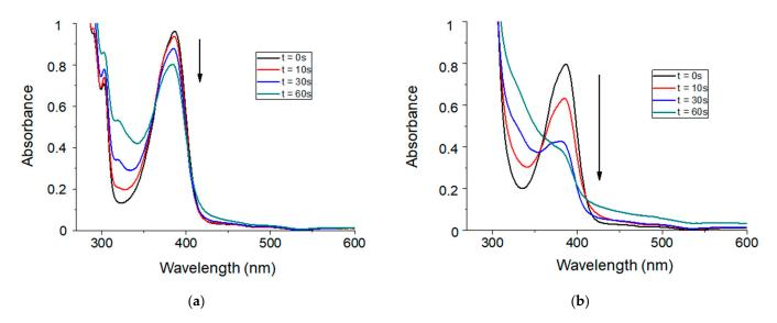
**Figure 1.** Steady-state photolysis in chloroform during 60 s of irradiation under LED@405 nm (100 mW/cm<sup>2</sup>) of (a) TXS alone and (b) TXS/Iod photoinitiating system. [TXS] =  $4.3 \times 10^{-3}$  mol/L, and [Iod] =  $8.6 \times 10^{-3}$  mol/L.
