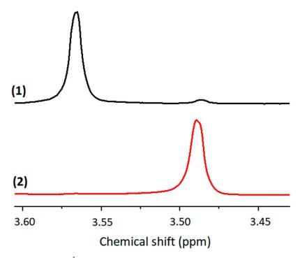
**Figure 5.** Liquid  $^{1}$ H NMR of the TXS/Iod solution in CDCl<sub>3</sub> before (1) and after (2) LED@385 nm irradiation (10 min, 130 mW/cm<sup>2</sup>).
