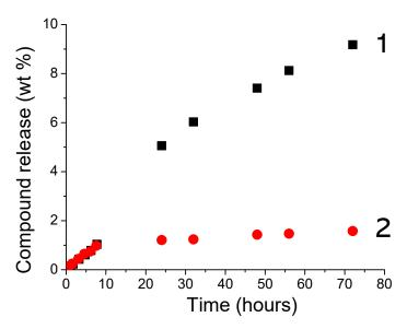
**Figure 9.** Release of TX (1) and TXS (2) from the photoinduced-GPTMS 25wt%/EPOX 75 wt% materials after 15 min under LED@405 nm irradiation (100 mW/cm<sup>2</sup>).
