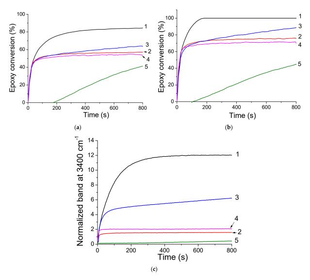
**Figure 8.** Evolution of the epoxy conversions of (a) DPDO and (b) GPTMS in the DPDO/GPTMS mixture, and (c) hydrolysis extent vs. irradiation time of GPTMS 25 wt%/DPDO 75 wt% formulation with TXS/Iod  $(1\%/2\% \ w/w)$  at LED@385 nm (1) under air, (2) in laminate at LED@405 nm, and (3) under air, (4) in laminate, and (5) at LED@455 nm under air.
