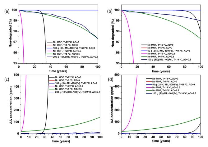
**Fig. 3.** Effect of temperature and MOF presence on a fresh film (AD=0, or initial acetic acid =0) as well as severely degraded film (AD=2.5, or initial acetic acid = 19 ppm). The degradation kinetics are reported where the film is stored at (a)  $T = 22^{\circ}$ C, (b)  $T = 16^{\circ}$ C. The acetic acid concentration in the atmosphere is reported for (c)  $T = 22^{\circ}$ C, (d)  $T = 16^{\circ}$ C.
