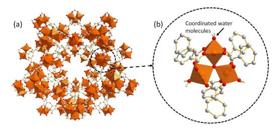
**Fig. 1.** MIL-100(Fe) structure with (a) a view of the large cage, (b) A close-up of the structure which is made up of iron trimers with open metal sites. Acetic acid adsorbs to MIL-100(Fe) in the presence of moisture due to its ability to displace coordinated water molecules [16]. Iron polyhedra, oxygen and carbon atoms are in orange, red and grey, respectively; hydrogen atoms have been omitted for the sake of clarity.
