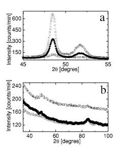
FIG. 1. X-ray-diffraction patterns measured in (a)  $\theta/2\theta$  and (b) GIS geometries on glass/Ta<sub>5</sub>/Py<sub>10</sub>/IrMn<sub>20</sub>/Py<sub>5</sub>/Ta<sub>5</sub> ( $\bigcirc$ ), glass/Ta<sub>5</sub>/Py<sub>10</sub>/IrMn<sub>20</sub>/Co<sub>5</sub>/Ta<sub>5</sub> ( $\bigcirc$ ), and glass/Ta<sub>5</sub>/Co<sub>10</sub>/IrMn<sub>20</sub>/Co<sub>5</sub>/Ta<sub>5</sub> ( $\square$ ) multilayers.
