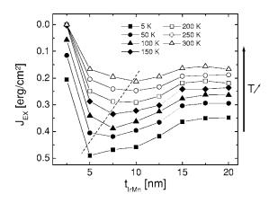
FIG. 3. Surface exchange coupling energy  $J_{\rm EX}$  evaluated from equation  $J_{\rm EX} = H_{\rm EX} M_S t_{\rm FM}$  for the top IrMn interface in glass/Ta<sub>5</sub>/Co<sub>10</sub>/IrMn<sub>t<sub>IrMn</sub></sub>/Co<sub>5</sub>/Ta<sub>5</sub> multilayers at temperatures from 5 to 300 K.
