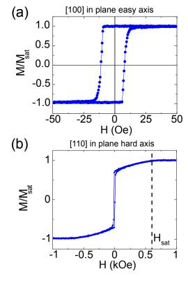
FIG. 11: M vs H measurements on a 10 nm thick Fe film for the easy [100] (a) and hard [110] (b) crystallographic axis. The saturation field  $(H_{sat})$  for the easy axis is around 10 Oe, while for the hard direction it reaches up to 600 Oe.
