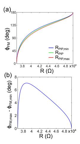
FIG. 10: (a)  $\Phi_{FM}$  as a function of resistance for the fittings with maximum, usual, and minimum  $R_{PIP}$  used, in the P-AP resistance range. (b) difference of calculated angle vs resistance (in the P-AP resistance range) for the fittings with maximum and minimum  $R_{PIP}$  used.
