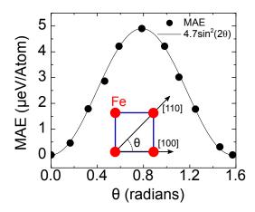
FIG. 12: Ab-initio calculation of magnetocryscalline anisotropy energy (MAE) as a function of the in-plane orientation angle  $\theta$ , defined in the inset. Solid line is a phenomenological fit to a  $\sin^2(2\theta)$  function.
