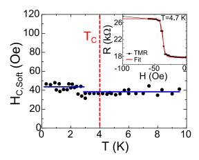
FIG. 8: Typical temperature dependence of the coercitive field of the soft Fe(001) ferromagnetic layer measured along [100] direction. The critical temperature is marked with a dashed red line. Blue lines are guides for the eye. The inset shows the method for determining the coercive field: a logistic fit was performed for the transition, and the coercive field was defined as the mid-height value of the fit.
