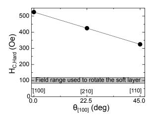
FIG. 6: Coercive field of the hard Fe/Co layer for magnetic field oriented along different crystallographic directions [100], [110] and [210], above the superconducting critical temperature ( $T=5~\mathrm{K}$ ). The grey band shows the typical field range used to manipulate the magnetization of the soft Fe(100) layer in the rotation experiments.
