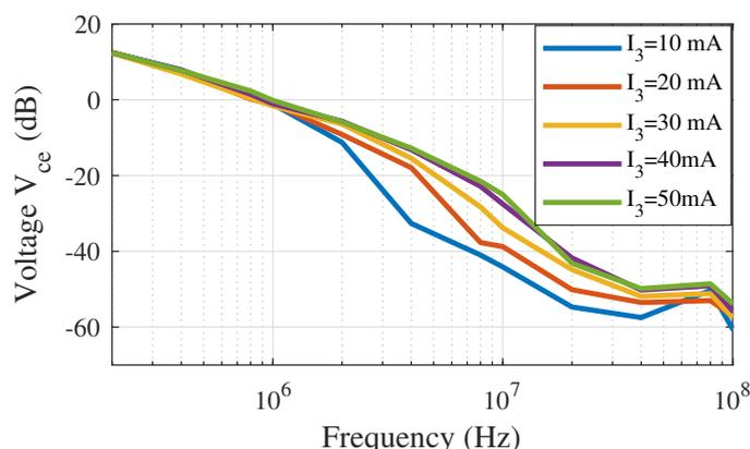
Fig. 7: Frequency spectra at different levels of  $I_3$ .Table II: Power losses for different level of  $I_3$
