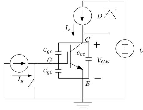
Fig. 4: Test circuit for the CSP evaluation.
