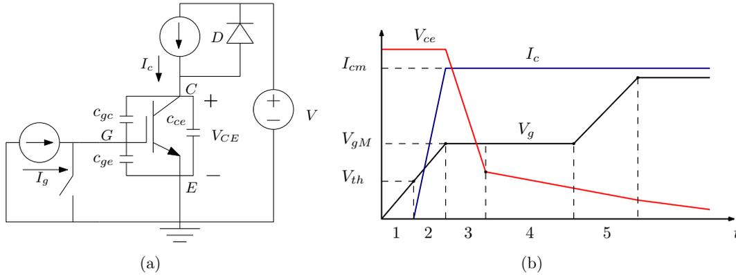
Fig. 2: (a) Test circuit and (b) dynamic charge during a turn-on transient.
