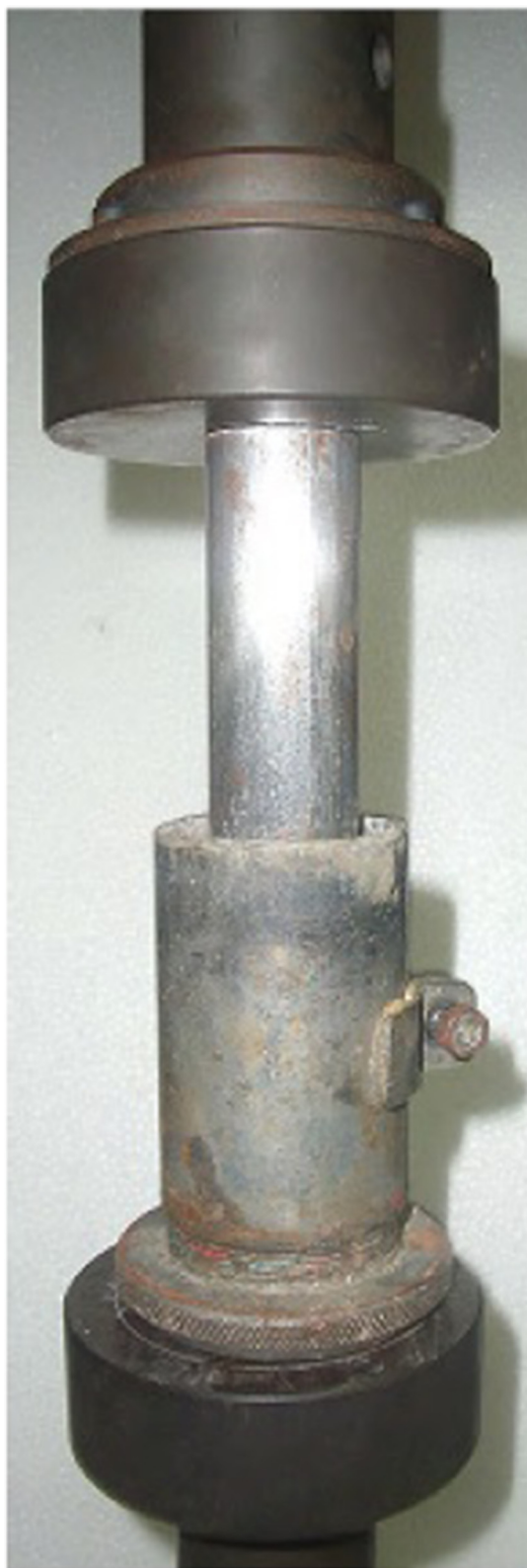
Figure 2 Specimen during the static push-out test.
