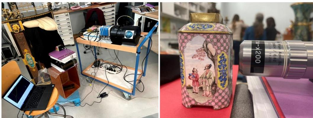
**Figure 1.** On-site Raman analysis: top, HE532 Horiba Jobin Yvon coupled with 532 nm Ventus laser and SuperHead® equipped with a ULWD 200X Mitutoyo microscope objective (bottom, zoom).
