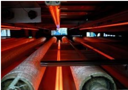
Heat tempering of flat glass
