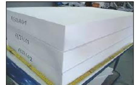
Insulating ceramic plates made of alumina (thickness : 100mm) [M. Schumann & L. San-Miguel, 2017]
