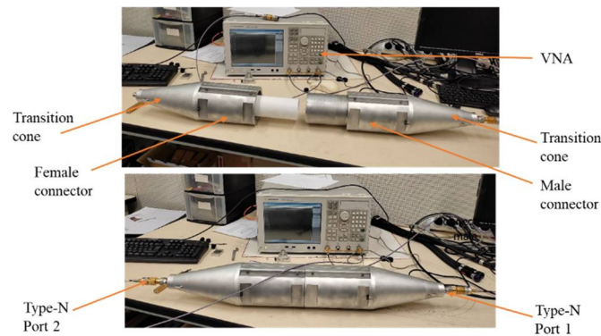
Figure 9. S-parameter measurement setup for transition cones and high-voltage connectors.
