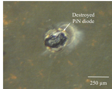
Fig. 9b. PI-passivated PiN diode after the breakdown at 7300 V (performed in PFPE environment).
