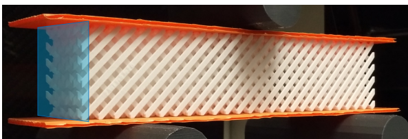
Figure 1: Example of pantographic block cross-section
