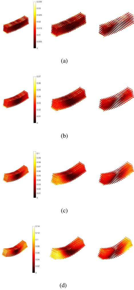
**Figure 20:** Maximum principal strain fields shown for the 4 different deformed configurations on the whole mesh (left), first family of beams (center) and second family of beams (right). (a) 5 mm, (b) 10 mm, (c) 15 mm and (d) 20 mm deflections
