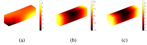
**Figure 9:** Displacement fields in the  $x$  (*i.e.*, longitudinal) (a),  $y$  (*i.e.*, transverse) (b) and  $z$  (*i.e.*, vertical) (c) directions obtained by the backtracking procedure. The fields are shown on the deformed configuration and expressed in voxels ( $1 \text{ vx} \equiv 0.1 \text{ mm}$ )
