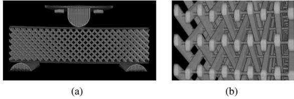
**Figure 2:** (a) 3D rendering of the studied metamaterial (length: 203.5 mm, height: 43.5 mm) with a  $100 \mu\text{m} / \text{vx}$  resolution. (b) Side view of hinges (0.90 mm in diameter) and beams
