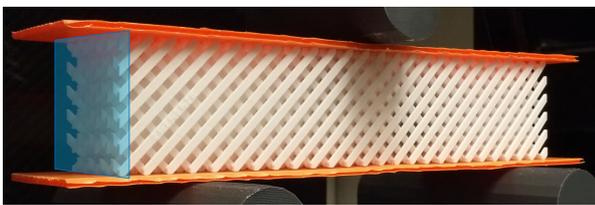
**Figure 1:** Example of pantographic block cross-section
