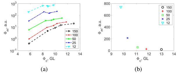
**Figure 14:** (a) Equilibrium gap  $\Phi_m$  vs. gray level residual  $\Phi_c$  for the five analyzed scans and for different regularization lengths (expressed in voxels,  $1 \text{ vx} \equiv 0.1 \text{ mm}$ ). (b) Corresponding plot for the last deformation step. The digitization of the registered volumes was 8 bits
