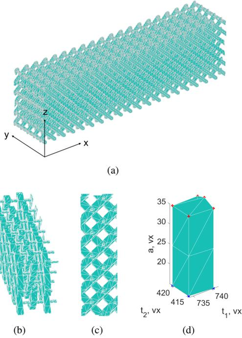
**Figure 7:** (a) Mesoscale mesh of the nominal configuration with its reference frame. Side (b) and front (c) views of hinges. (d) Detail of one individual hinge and its reference frame (axial and tangential directions). The red and blue nodes depict the top respectively the bottom planes used to measure displacement and rotation jumps
