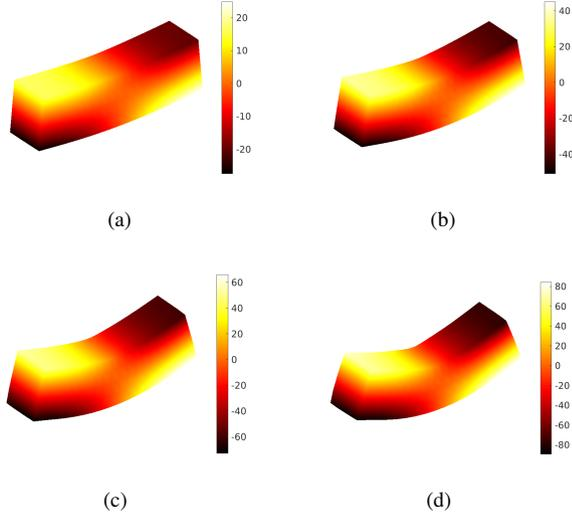
**Figure 13:** Initialization results in terms of displacements (expressed in voxels,  $1 \text{ vx} \equiv 100 \mu\text{m}$ ) along the  $x$  (*i.e.*, longitudinal) direction for the different deformed configurations. (a) 5 mm, (b) 10 mm, (c) 15 mm and (d) 20 mm deflections
