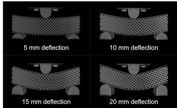
**Figure 4:** 3D renderings of the 4 deformed configurations
