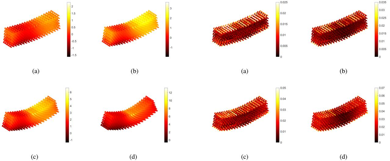
**Figure 18:** Displacement fields along the  $y$  (*i.e.*, transverse) direction for the different deformed configurations. (a) 5 mm, (b) 10 mm, (c) 15 mm and (d) 20 mm deflections. The displacements are expressed in voxels ( $1 \text{ vx} \equiv 0.1 \text{ mm}$ )
