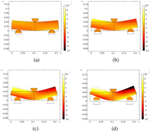
**Figure 28:** Computed longitudinal displacement fields on the deformed shapes of the pantographic block for different prescribed deflections: (a) 5 mm, (b) 10 mm, (c) 15 mm and (d) 20 mm. The displacements are expressed in mm.
