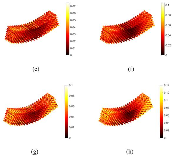
**Figure 19:** Von Mises equivalent strain (left) and maximum principal strain (right) fields for the 4 different deformed configurations. (a,b) 5 mm, (c,d) 10 mm, (e,f) 15 mm and (g,h) 20 mm deflections
