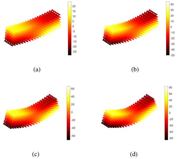
**Figure 17:** Displacement fields along the  $x$  (*i.e.*, longitudinal) direction for the different deformed configurations. (a) 5 mm, (b) 10 mm, (c) 15 mm and (d) 20 mm deflections. The displacements are expressed in voxels ( $1 \text{ vx} \equiv 0.1 \text{ mm}$ )
