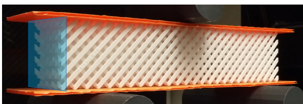
Figure 1: Example of pantographic block cross-section
