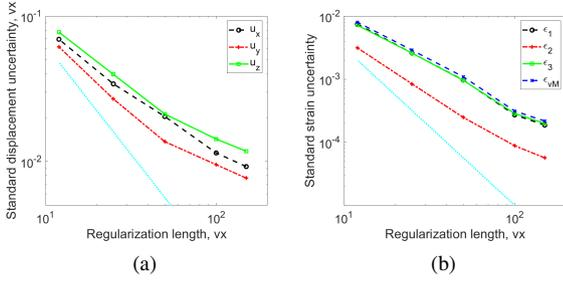
**Figure 10:** Standard displacement (a) and strain (b) uncertainties as functions of the regularization length  $\ell_m$ . The physical size of one voxel is 0.1 mm. The cyan dotted lines show power law interpolations with exponents  $-3/2$  (a) and  $-5/2$  (b)
