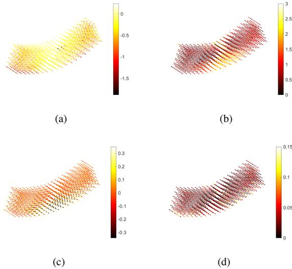
**Figure 23:** Axial (a) and transverse (b) displacement jumps (expressed in voxels,  $1 \text{ vx} \equiv 0.1 \text{ mm}$ ) for each hinge. Corresponding axial (c) and transverse (d) rotation jumps (expressed in rad) for each hinge. The results are shown for the last deformed configuration
