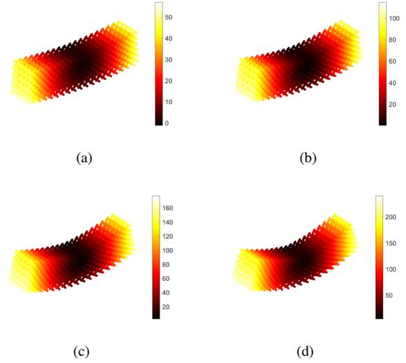
**Figure 16:** Displacement fields along the  $z$  (*i.e.*, vertical) direction for the different deformed configurations. (a) 5 mm, (b) 10 mm, (c) 15 mm and (d) 20 mm deflections. The displacements are expressed in voxels ( $1 \text{ vx} \equiv 0.1 \text{ mm}$ )
