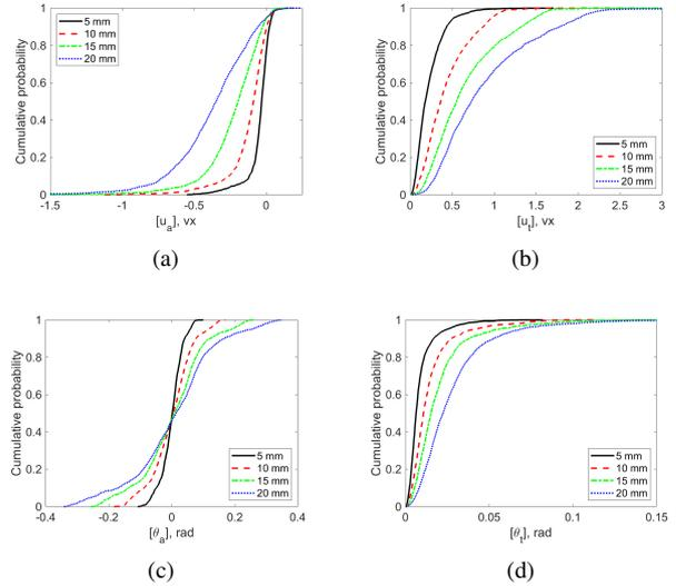
**Figure 24:** Cumulative plots of axial (a) and transverse (b) displacement jumps for the four applied deflections. The displacements are expressed in voxels ( $1 \text{ vx} \equiv 0.1 \text{ mm}$ ). Corresponding plots for the axial (c) and transverse (d) rotation jumps
