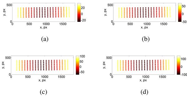
**Figure 21:** Vertical displacement fields  $u_z$  of each hinge center of gravity (of the upper row of the pantographic block) once the rigid body motions were subtracted. (a) 5 mm, (b) 10 mm, (c) 15 mm and (d) 20 mm deflections. The displacements are expressed in voxels ( $1 \text{ vx} \equiv 0.1 \text{ mm}$ )
