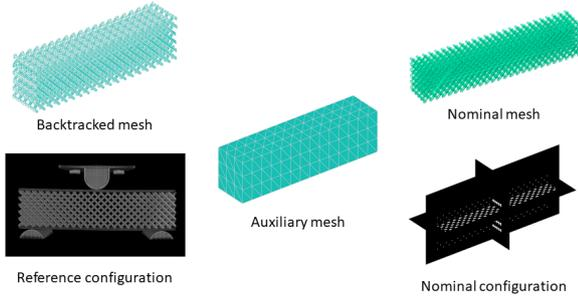
**Figure 8:** Reference (printed) configuration to be registered with the nominal configuration via DVC using an auxiliary (*i.e.*, macroscopic) mesh encompassing the reference configuration. The nominal mesh is then backtracked
