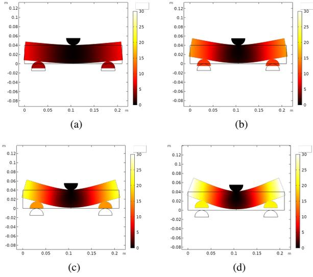
**Figure 27:** Computed transverse displacement fields on deformed shapes of the pantographic block for different prescribed deflections: (a) 5 mm, (b) 10 mm, (c) 15 mm and (d) 20mm. The displacements are expressed in mm.
