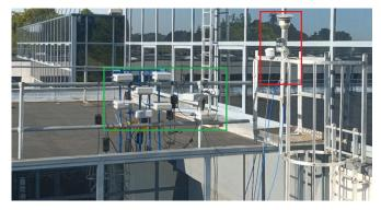
Figure 1: The experimental setup containing the 12 sensors (framed by green) and reference instrument measurement (sampling  $PM_{2.5}$  framed by red).
