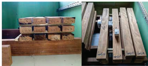
Figure 6: Natural drying tests: left, D. guianensis ; right, 8 wood elements ( D. guianensis and Q. rosea ) equipped with sensors.
