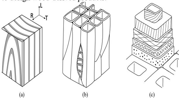
Figure 1: Hierarchical structure and anisotropy of wood
