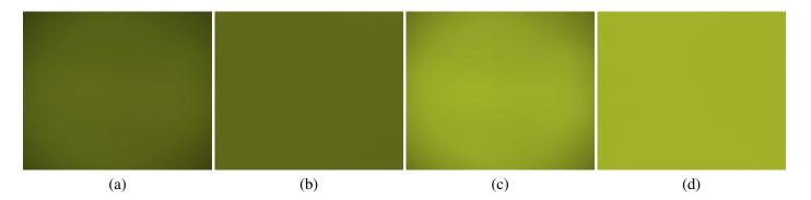
Figure 10: Calibration effects over a uniform, linearly polarized light, with an AoLP of  $40^{\circ}$ . These images are the demosaiced, RGB polarization channels. (a) and (c) Uncalibrated polarization channels  $0^{\circ}$  and  $45^{\circ}$ , respectively. (b) and (d) Calibrated polarization channels  $0^{\circ}$  and  $45^{\circ}$ , respectively.
