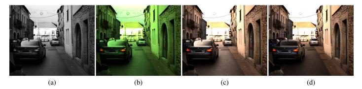
Figure 7: (a) Raw, mosaiced version of the reference image, for the polarization channel  $0^{\circ}$ . (b) Demosaiced version of the reference image, without white-balance, for the  $0^{\circ}$  polarization channel. (c) White-balanced, demosaiced images for the polarization channel  $0^{\circ}$ . (d) White-balanced, demosaiced images for the polarization channel  $135^{\circ}$ .
