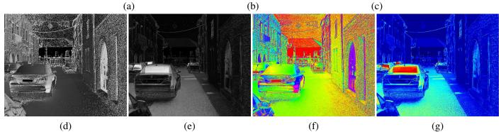
Figure 8: Polarization images for the red channel. (a) (b) (c)  $S_{0,1,2}$  components of the Stokes vector. The parameter  $S_0$  corresponds also to the total intensity image. (d) (e) Raw AoLP, and Raw DoLP. (f) Raw AoLP of the red channel, colored with the HSV palette. (g) Raw DoLP of the red channel, colored with the Jet palette.
