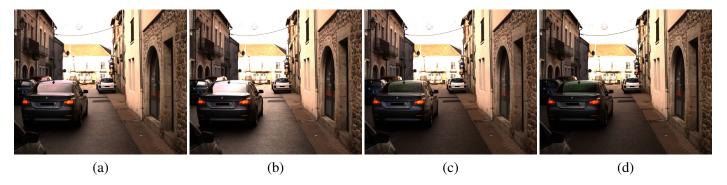
Figure 13: Specularity removal application results. (a) Unfiltered, total intensity. (b) (c) Filtered image by simulating a linear polarization filter oriented at  $60^{\circ}$ , and  $120^{\circ}$ , respectively. (d) Polarized specularity removal by filtering with the degree of linear polarization.
