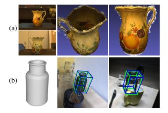
Figure 5: Results of some of the reviewed algorithms for pose estimation. From left to right: (a) Input RGB image, reconstructed surface with the algorithm provided in [12]. (b) Glass vase model, and the detected pose from two view-points. Results courtesy of [53].
