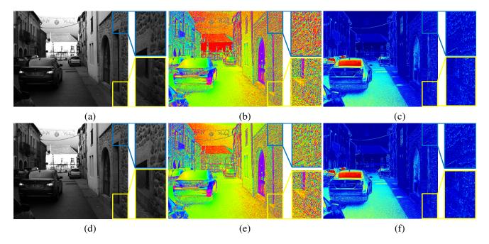
Figure 12: Calibration effects over the polarization images, for the red channel. Top row: uncalibrated images. Bottom row: calibrated images. (a) (d) Total intensity. (b) (e) Angle of linear polarization, colored with the HSV palette. (c) (f) Degree of linear polarization, colored with the Jet palette.
