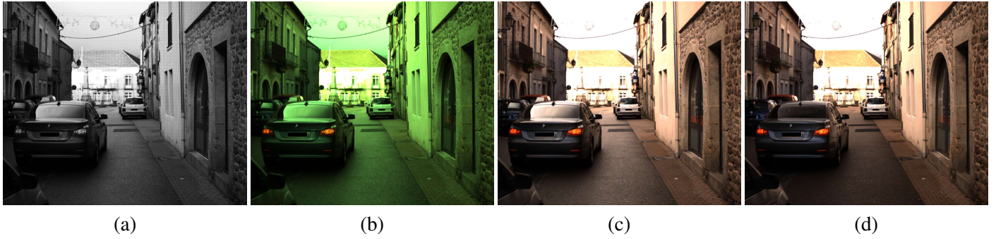
Figure 7: (a) Raw, mosaiced version of the reference image, for the polarization channel 0^\circ . (b) Demosaiced version of the reference image, without white-balance, for the 0^\circ polarization channel. (c) White-balanced, demosaiced images for the polarization channel 0^\circ . (d) White-balanced, demosaiced images for the polarization channel 135^\circ .
