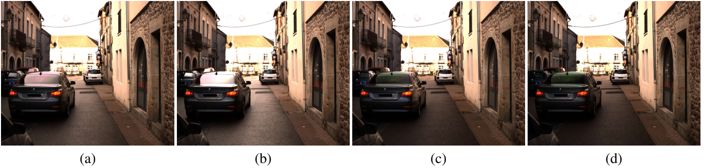
Figure 13: Specularity removal application results. (a) Unfiltered, total intensity. (b) (c) Filtered image by simulating a linear polarization filter oriented at 60^\circ , and 120^\circ , respectively. (d) Polarized specularity removal by filtering with the degree of linear polarization.
