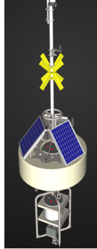
Fig. 11: Schematic diagram of the buoy with mast. The keel is weighted to balance the buoyancy
