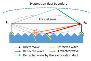
Fig. 2: Radio wave propagation near the sea surface
