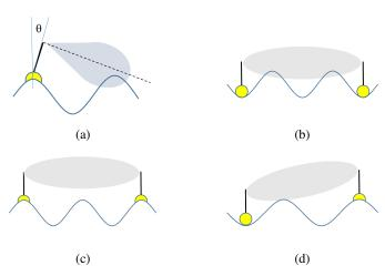
Fig. 7: Influence of the waves: a) On the signal propagation direction; b-d) Interaction between the Fresnel zone and waves vs buoy position
