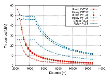
Fig. 16: Throughput of different packet size payloads in SF7, with the relay node placed 2km away from the gateway to consider the sensitivity of SF7.
