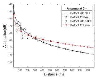
Fig. 5: Attenuation versus distance at 433MHz using a Petool model in the case of transmission over the sea or over a lake, for an antenna height  $h_{\text{Ant}}=2\text{m}$  with an aperture angle of  $20^{\circ}$  or  $1^{\circ}$
