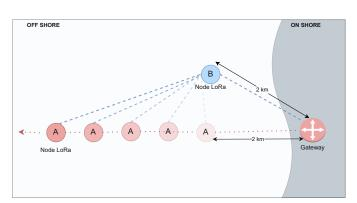
Fig. 12: Node A transmits data at varying distances from the gateway, gradually increasing the distance between them in order to evaluate the impact of distance on the strength and quality of the wireless signal.
