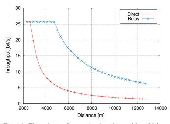
Fig. 14: Throughput of transmitted packets with a 23-byte payload in SF7.
