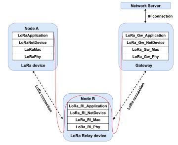
Fig. 13: LoRaWAN relay node process for forwarding packets
