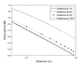
Fig. 6: Attenuation versus distance at 433MHz for different antenna heights using a Petool model
