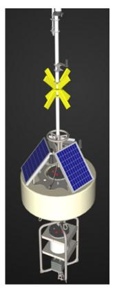
Fig. 11: Schematic diagram of the buoy with mast. The keel is weighted to balance the buoyancy
