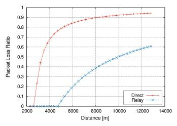
Fig. 15: Packet loss ratio of transmitted packets with a 23-byte payload in SF7.
