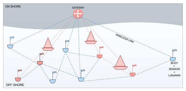
Fig. 1: Each buoy is equipped with a LoRaWAN node. Nodes marked in red cannot transmit directly to the gateway due to ships causing interference between the node and the gateway. Thus, they require relaying on buoys marked in blue to reach the gateway.
