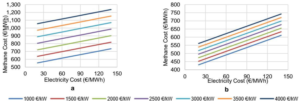
Figure 4: Impact of Electricity cost (€/MWh) and the cell capital cost (€/kW) on the final methane cost (€/MWh) at a fixed maximum CO<sub>2</sub> cost of 100 €/t, and two different cell lifetimes: 10,000 h (a), and 40,000 h (b)
