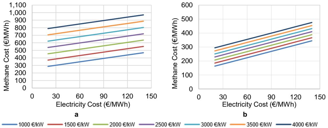
Figure 3: Impact of Electricity cost (€/MWh) and the cell capital cost (€/kW) on the final methane cost (€/MWh) at a fixed minimum CO<sub>2</sub> cost of 20 €/t, and two different cell lifetimes: 10,000 h (a), and 40,000 h (b)
