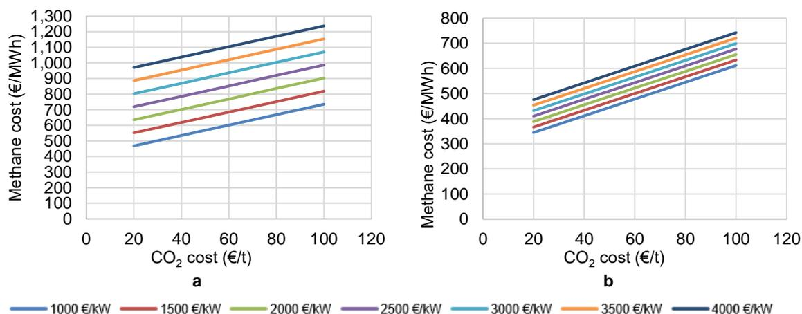
Figure 2: Impact of CO<sub>2</sub> feed cost (€/t) and the cell capital cost (€/kW) on the final methane cost (€/MWh) at a fixed electricity cost of 140 €/MWh, and two different cell lifetimes: 10,000 h (a), and 40,000 h (b)
