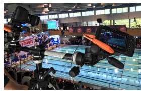
Fig. 5: Video recording setup: left and right cameras independently recorded half of the pool.
