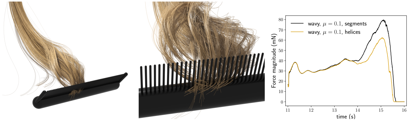
Fig. 1. A wavy hair wisp made of 2025 super-helices is virtually combed, yielding a hundred thousand tight frictional contacts ( \mu = 0.1 ). In this paper we show that during such a sliding motion, the force response is highly dependent on the proxy elements used for collision detection . In particular, we find that even in the case of a rod model with a C^1 -smooth centreline, segment-based collision detection yields artificial noise in the contact force response, which increases with the curvature of the rod at each contact point. We introduce a new detection scheme between two smooth curves that fixes this issue. Compared to a classical segment-based detection scheme (right plot, black curve), our method retrieves force profiles that integrate much less noise (yellow curve), hence increasing the accuracy of force prediction.
