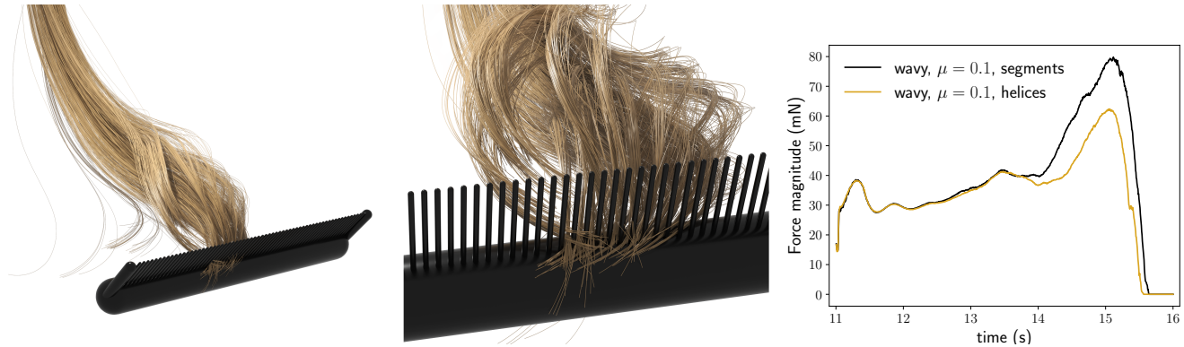
Fig. 1. A wavy hair wisp made of 2025 super-helices is virtually combed, yielding a hundred thousand tight frictional contacts ( \mu = 0.1 ). In this paper we show that during such a sliding motion, the force response is highly dependent on the proxy elements used for collision detection . In particular, we find that even in the case of a rod model with a C^1 -smooth centreline, segment-based collision detection yields artificial noise in the contact force response, which increases with the curvature of the rod at each contact point. We introduce a new detection scheme between two smooth curves that fixes this issue. Compared to a classical segment-based detection scheme (right plot, black curve), our method retrieves force profiles that integrate much less noise (yellow curve), hence increasing the accuracy of force prediction.
