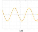
Fig 16. Measured line current output with m =0.6(20A/div., 5ms/div.).(a) CSVPWM. (b) R-ZVD-SVPWM. (c) Proposed SVPWM.
