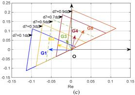
Fig 6. Different trajectories of the harmonic flux. (a) Different modulation index CSVPWM. (b) Different angles m=0.7 with CSVPWM. (c)Different ZVD m=0.7 and  $\theta$ =45°.
