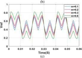
Fig 9. Phase voltage reference. (a) CVPWM. (b) R-ZVD-SVPWM. (c) Proposed SVPWM.
