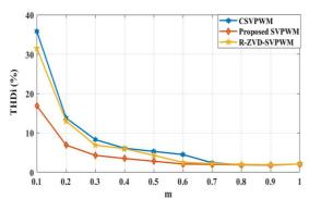
Fig 20. Measured phase current output THD.
