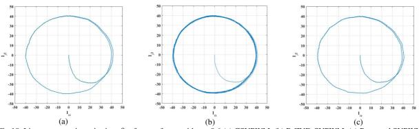
Fig 19. Line current trajectories in  $\alpha$ - $\beta$  reference frame with m = 0.6.(a) CSVPWM. (b) R-ZVD-SVPWM. (c) Proposed SVPWM.
