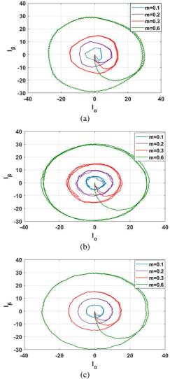
Fig 11. Line current trajectories in α-β plan reference frame.(a) CVPWM. (b) R-ZVD-SVPWM. (c) Proposed SVPWM.
