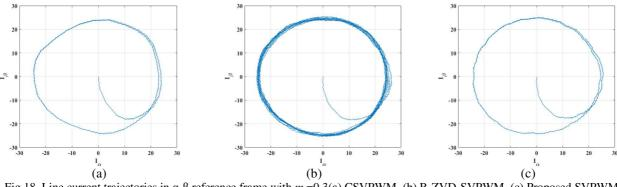
Fig 18. Line current trajectories in  $\alpha$ - $\beta$  reference frame with m =0.3(a) CSVPWM. (b) R-ZVD-SVPWM. (c) Proposed SVPWM.
