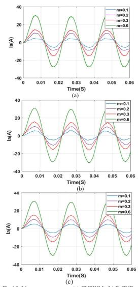
Fig 10. Line courant output. (a) CVPWM. (b) R-ZVD-SVPWM.(c) Proposed SVPWM.
