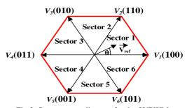
Fig 2. Space-vector diagram for the SVPWM.
