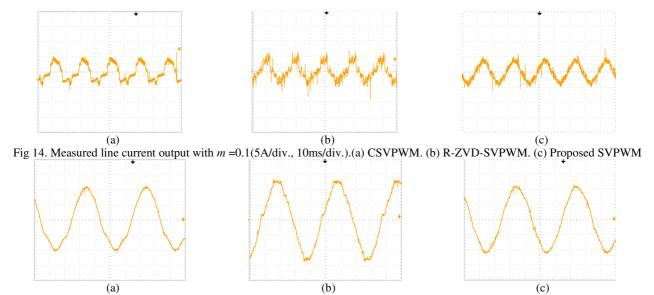
Fig 15. Measured line current output with m =0.3(10A/div., 5ms/div.).(a) CSVPWM. (b) R-ZVD-SVPWM. (c) Proposed SVPWM.
