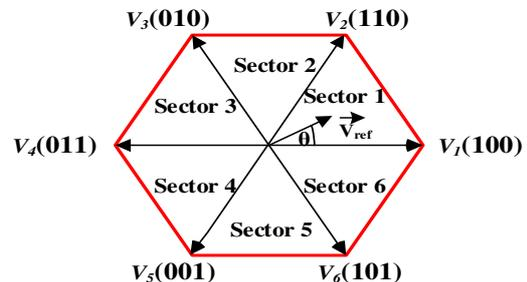
Fig 2. Space-vector diagram for the SVPWM.
