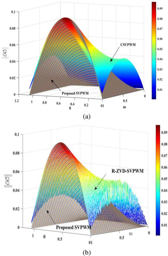
Fig 8. 3-D graphical presentation of the gravity center displacement. (a) CSVPWM and the proposed SVPWM. (b) R-ZVD-SVPWM and the proposed SVPWM.
