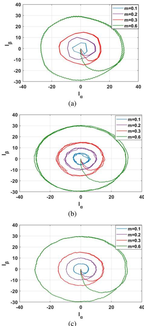
Fig 11. Line current trajectories in  $\alpha$ - $\beta$  plan reference frame.(a) CVPWM. (b) R-ZVD-SVPWM. (c) Proposed SVPWM.
