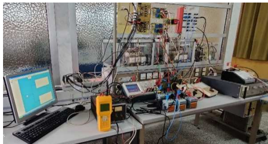
Fig 13. Photography of the experimental test bench.
