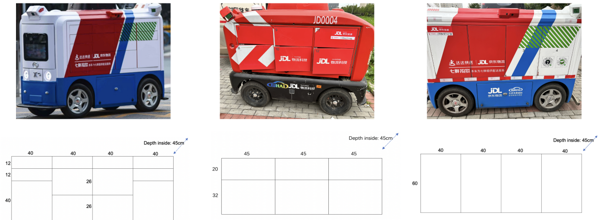
Figure 9 The three types of robots considered by JD.com: Type 1 (left), Type 2 (middle), and Type 3 (right)
