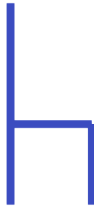
Figure 4: Chair shaped well with one junction and four branches of sizes 600 m (upper vertical branch), 400 m (lower left vertical branch), 400 m (lower vertical branch) and 400 m (horizontal branch).
