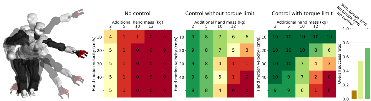
Figure 7. Comparison of our controller’s robustness against model errors and motion velocity. The Talos robot performs in double support 10 far-reaching tasks at the edge of the feasibility boundary in the MuJoCo simulator (left). The number of successful trials without falling is indicated (out of 10). Different combinations of hand motion velocity and added mass on the robot’s hand are compared (middle). The comparison includes scenarios with the SEIKO controller disabled (only open-loop SEIKO retargeting), the SEIKO controller with only foot wrenches control, and the full controller also considering joint torque limits. Overall success ratio comparing the three controllers is given on right panel.
