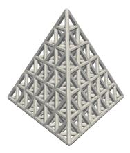
Figure 3: CAD model of the tetrahedral lattice material
