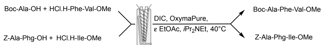
Scheme 2. Two examples of tripeptides synthesized by reactive extrusion
