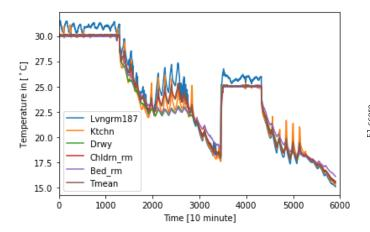
Fig. 2: The temperature evolution in different rooms of the Twin House. The data corresponding to Lvngrm187, Ktchn, Drwy, Chldrrm, Bedrm are the temperature data from the living room, kitchen, doorway and bedroom temperature sensors, respectively. Tmean is the average temperature of all rooms.
