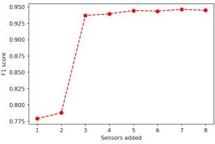
Fig. 4: Accuracy with increasing number of sensors.
