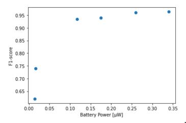
Fig. 5: Trade-off between accuracy and battery power consumption with optimized sensor configurations.
