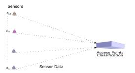
Fig. 1: Overview of the sensing and communication infrastructure for condition-based maintenance. Sensors collect data and, depending their configuration, compress and communicate the data to an access point. The access point identifies anomalies via a classifier tailored to the sensor configurations.
