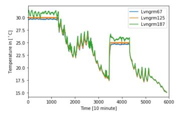
Fig. 3: Temperature measured in the same room with sensors at different heights in living room of the Twin House. Lvngrm67, Lvngrm125, Lvngrm187 is the temperature data from the sensors at the height of 1.25 m, 1.67 m and 1.87 m, respectively [39]).
