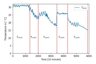
Fig. 9: The sectioning of twin house data in different zones (dashed vertical lines), each zone has a different cost function defined by penalties  $\lambda_{t,1}$ ,  $\lambda_{t,2}$  and different temperature limits for anomaly detection.
