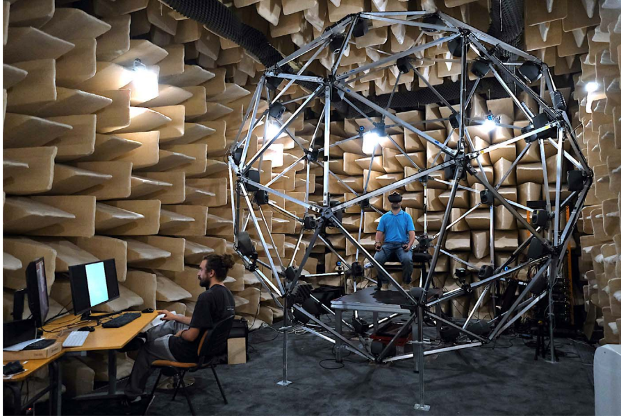
Figure 3. Spatialization system at PRISM Laboratory (Marseille, France). It consists of a spherical array of 42 loudspeakers (Genelec 8020C) with a diameter of 3.8 m, situated in a semi-anechoic chamber. Auralization is performed by a 4th order HOA rendering (decoder: energy-preserving with basic optimization) of SRIRs measured with mh-acoustics em32.
