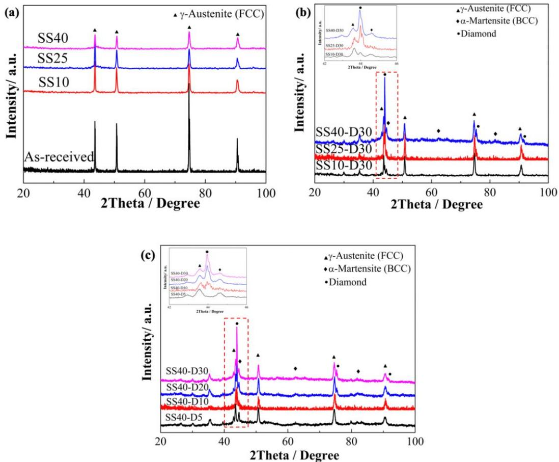
**Fig. 4.** XRD patterns of the SS 316 substrates (a) before and after fs-laser texturing with microgrid depths of 10, 25 and 40  $\mu\text{m}$ , respectively; (b) with diamond coatings on the 10, 25 and 40  $\mu\text{m}$  microgrids, respectively; (c) with diamond coatings on the 40  $\mu\text{m}$  microgrid for deposition periods of 5, 10, 20 and 30 min, respectively.
