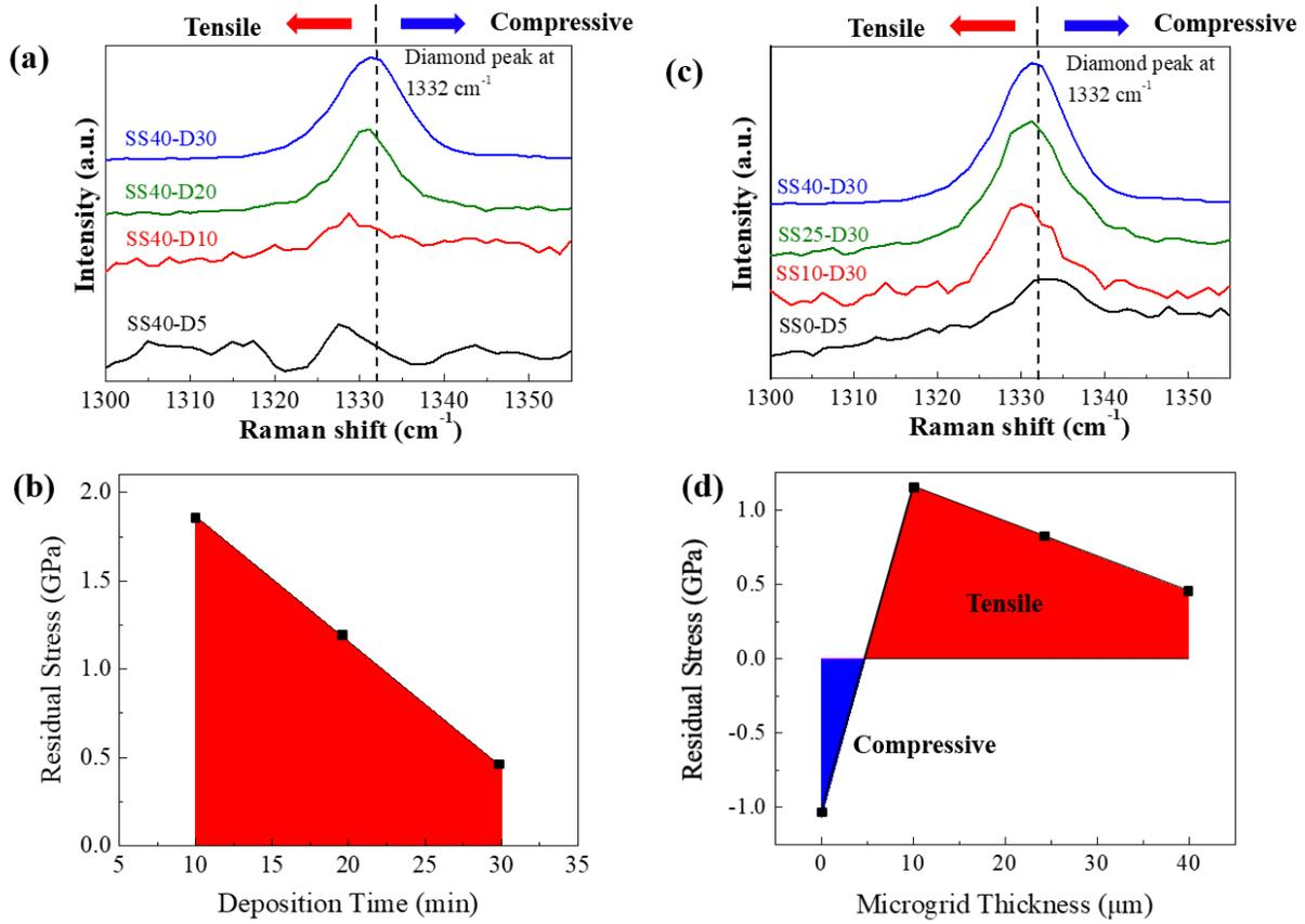
**Fig. 7.** Raman spectra near  $1332 \text{ cm}^{-1}$  and calculated residual stress of the diamond coatings deposited on the fs-laser textured SS 316 substrates (a), (b) after deposition from 5 to 30 min with the microgrid depth of 40  $\mu\text{m}$ ; (c), (d) with the microgrid depths of 10, 25, and 40  $\mu\text{m}$  after 30 min deposition.
