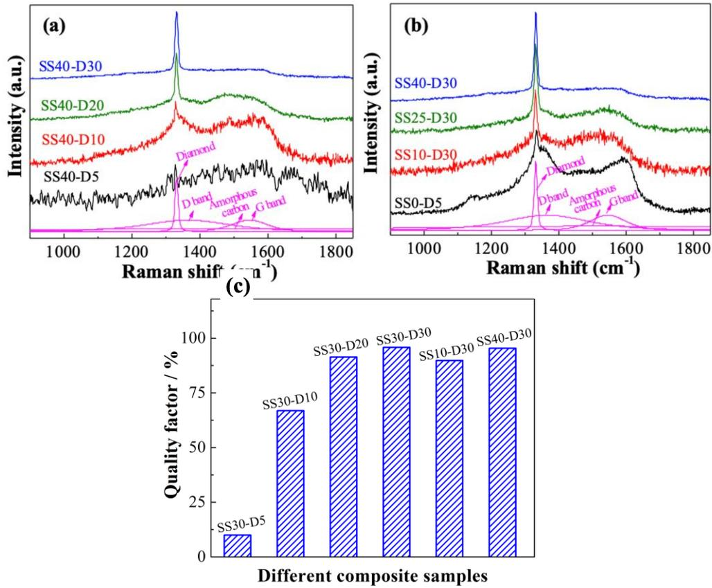
**Fig. 6.** Raman spectra of the diamond coatings deposited on the fs-laser textured SS 316 substrates (a) with a microgrid depth of 40  $\mu\text{m}$  after deposition times from 5 to 30 min, (b) with the microgrid depths of 0, 10, 25 and 40  $\mu\text{m}$  after 30 min of deposition, (c) the diamond quality factors calculated based on the Raman spectra.
