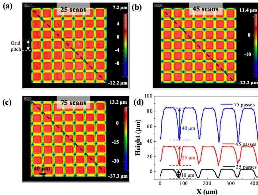
**Fig. 2.** Zygo mappings of the fs-laser textured SS 316 substrates with: (a)-(c) 25, 45 and 75 scanning passes. (d) diagonal profiles obtained from (a)-(c) as marked by the dashed lines.
